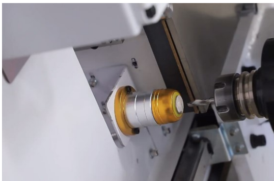
ATC linear tool changer magazines with 12 positions
